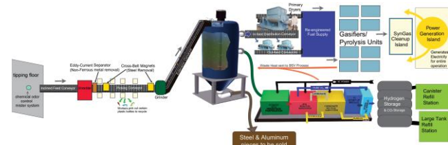
Figure 4: Total Recovery Facility.
