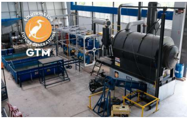
Semi-industrial pyrolysis by GTM - 800kg/ daily batch- (200 tonnes/year)
