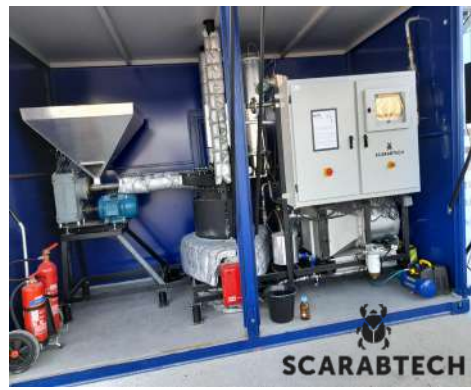
Containerized pyrolysis by Scarabtech - 20-40kg/h
