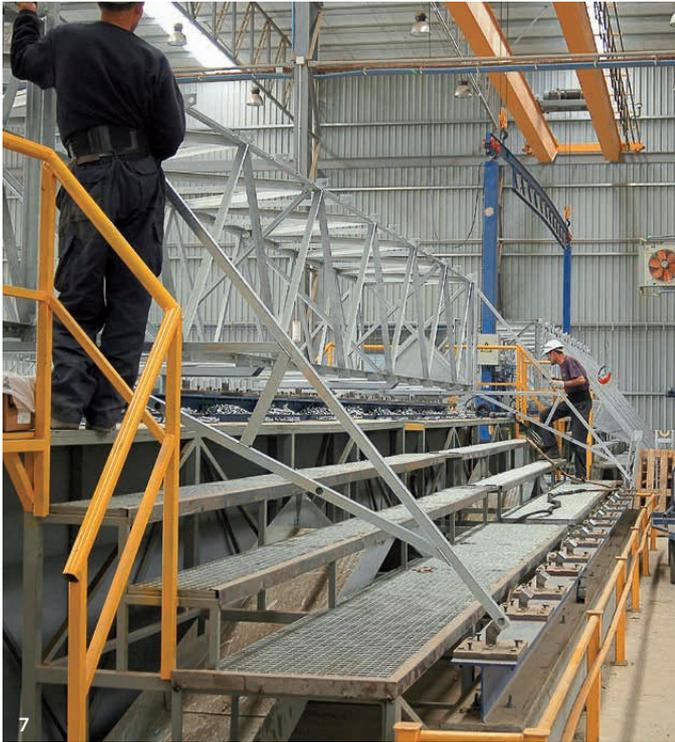
the steel construction industry. However, these tolerances are still far too large to achieve the necessary precision of the finished collector and hence the necessary optical quality.
