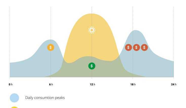
WATTS gives customer ability to shift electricity demand from peak to off-peak periods without the need for behavioural changes, by pre-charging during off-peak hours and discharging to meet customer load during peak periods. This control allows customers to minimize peak rate purchase, and should save them significant money in the long term.
