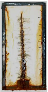
Panel II-91-10 – 9404 Hours Salt Fog Exposure (Scraped at 8372 Hours)
