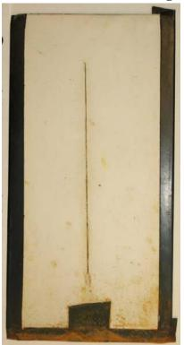
**Panel II-91-16** – **7404 Hours Salt Fog Exposure** Note that red corrosion products are contamination from an adjacent sample in the exposure cabinet and not corrosion of the substrate.
