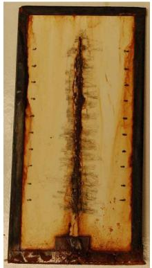
Panel II-91-6 – 11420 Hours Salt Fog Exposure (Scraped at 8372 Hours)
