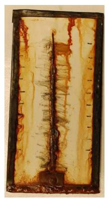
Panel II-91-10 – 11420 Hours Salt Fog Exposure (Scraped at 8372 Hours)
