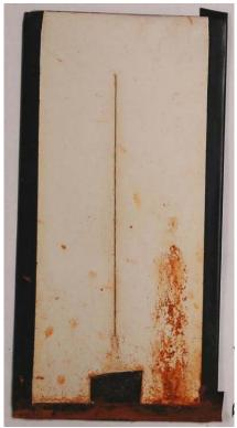
**Panel II-91-16** – **10740 Hours Salt Fog Exposure** Note that red corrosion products are contamination from an adjacent sample in the exposure cabinet and not corrosion of the substrate.
