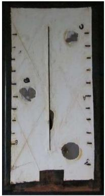
Panel II-91-2 – Following 8372 Hours Salt Fog Exposure and Adhesion Testing
