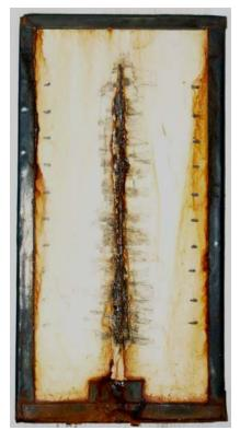
Panel II-91-6 – 9404 Hours Salt Fog Exposure (Scraped at 8372 Hours)
