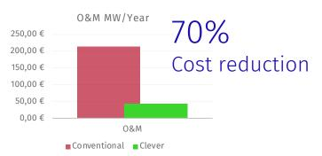
NOTE: This calculations have been made with 50€/KW cost, however CONVENTIONAL costs are highly dependent on electricity cost and rises exponentially when the price/KW goes up while Clever Solar Devices solutions remains unaffected.
