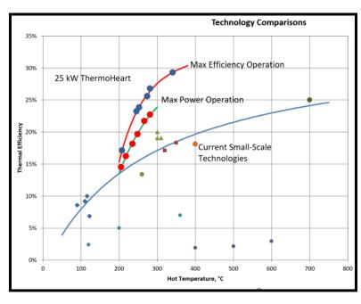
25kW ThermoHeart measured performance compared to
