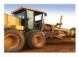
**3.** Mix applied ECOROADS treated material in a windrow using a grader blade or soil mixer. Blade treated soil mix to create road level and crown surface.
