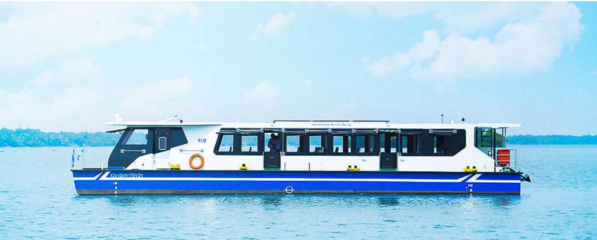
RIVEIERE is a catamaran ferry boat with a GRP (Glass Reinforced Plastic, also known as FRP, or Fiber Reinforced Plastic) hull and an aluminium superstructure built under IR Class (Indian Register of Shipping, a member of the International Association of Classification Societies).
