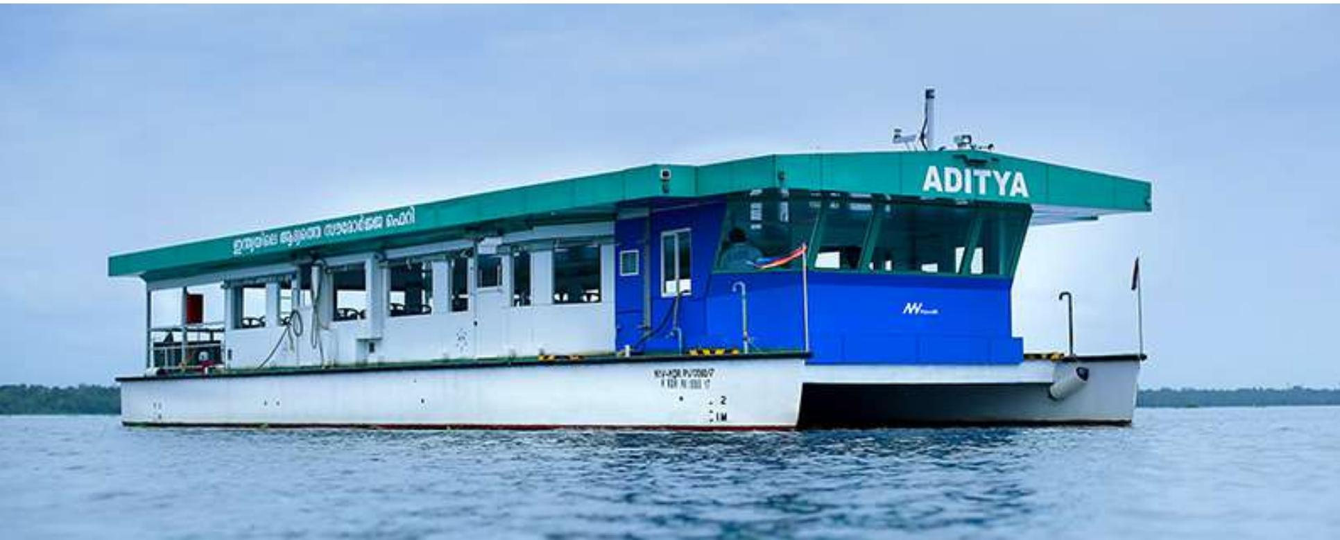
ADITYA is a catamaran ferry boat with a GRP (Glass Reinforced Plastic, also known as FRP, or Fiber Reinforced Plastic) hull and an aluminium superstructure built under IR Class (Indian Register of Shipping, a member of the International Association of Classification Societies).
