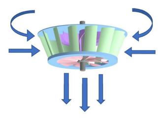
In a more efficient variant, another similar platform will rotate above this platform, but in the reverse mode of operation. It will rotate in the opposite direction. The upper propeller will grip the air and blow it through the side blades. **Thus, the upper platform will supply the bottom with a large amount of air.**
