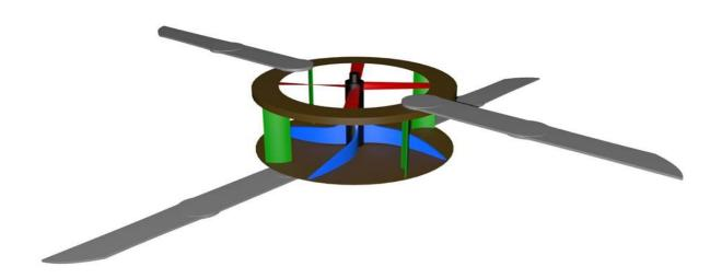
The turbo - propeller differs that its blades are mounted on a turbo - platform.
