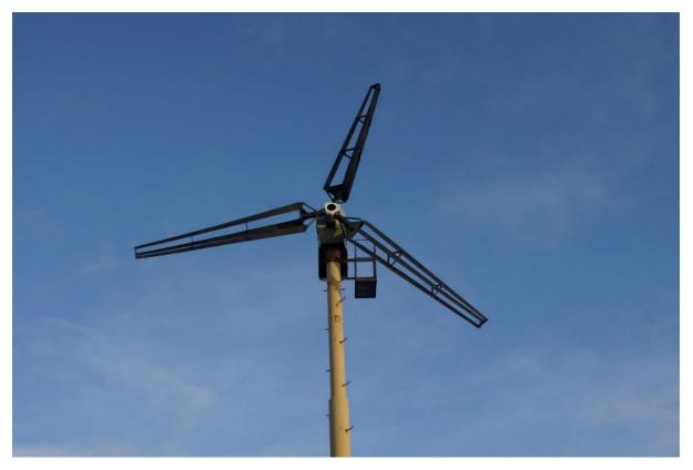
Pilot demonstration of a 7.4m diameter Triblade rotor on a test turbine.
