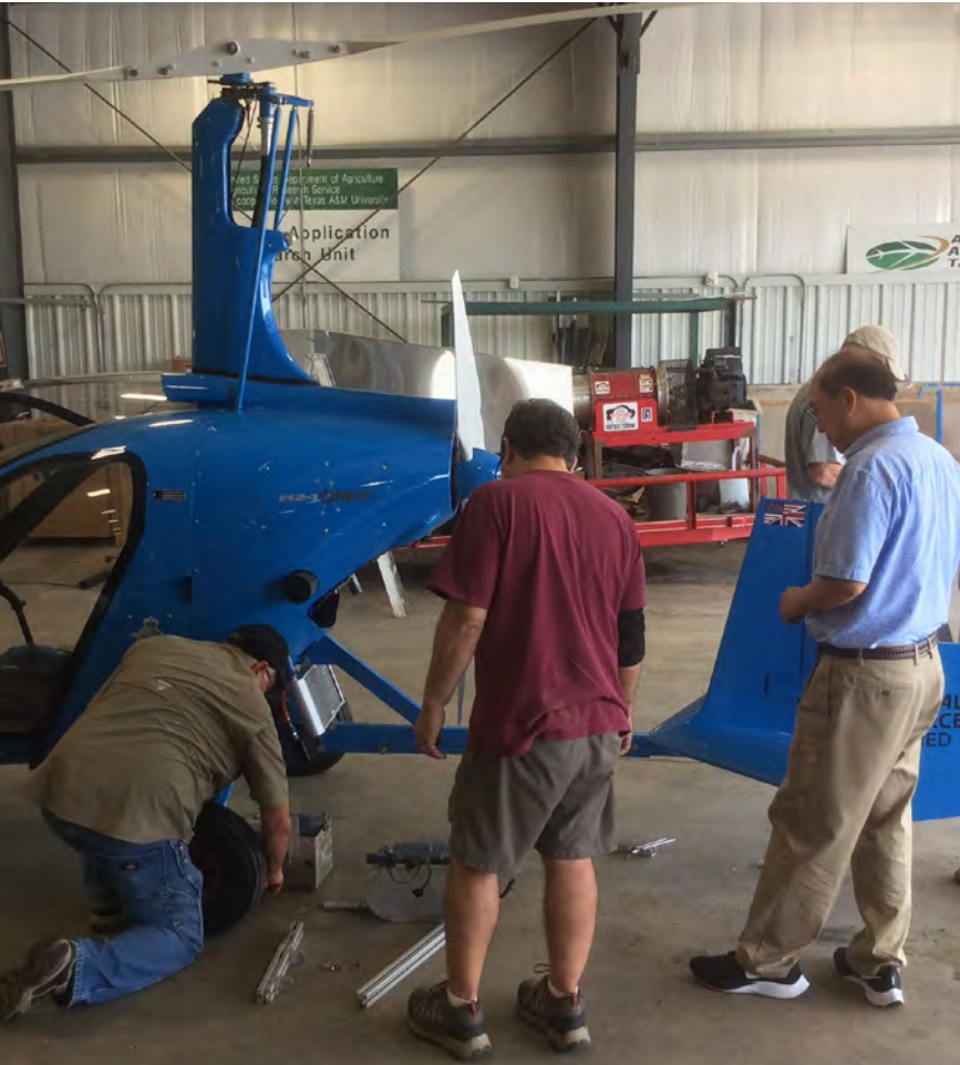
ATTACHING CAMERAS TO THE MAGNI GYROPLANE M24 (PHOTO COURTESY JONATHAN SCOTT)
